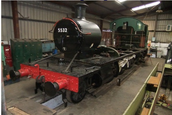
5532 new smokebox and door fitted 2016
